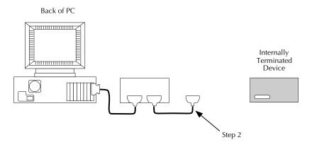
3. Position the Scanner so that you can connect it in the chain before the terminated device.
